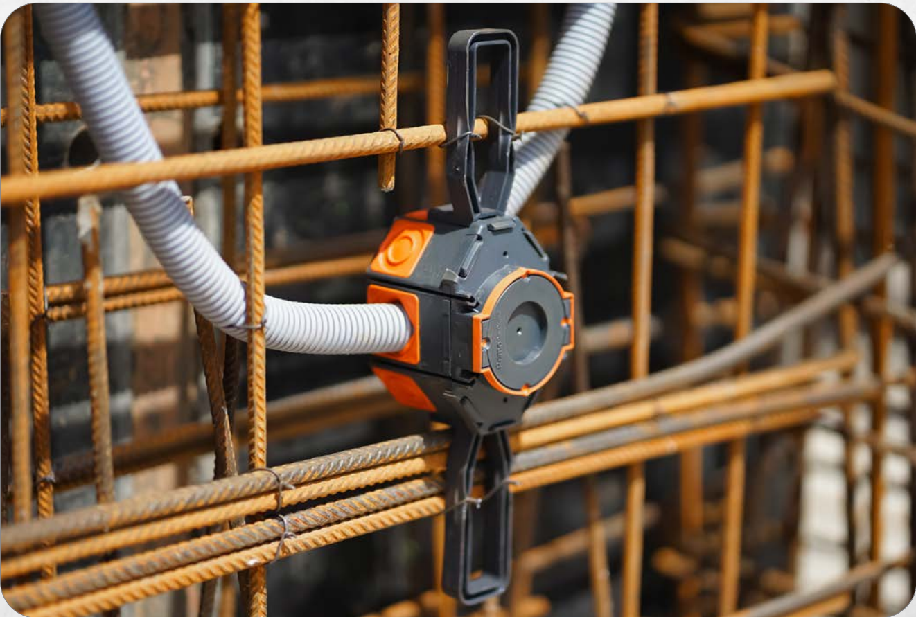
1. Push Wings onto the membrane box M1, M2 or M3. Wings set the 15 cm standard distance to door formwork and enable easy mounting. Fasten the Wings to the steel reinforcement with wire.
