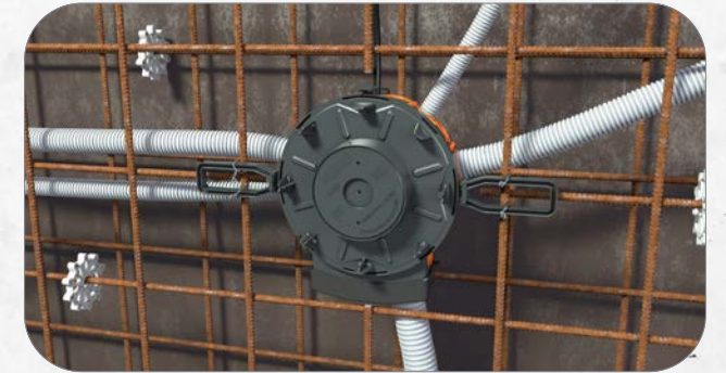
2. Open the membrane with a cutter knife. Combination entry of cables and (rigid) conduits from M9 - M40 without tools. The membrane technology guarantees absolute concrete-tight entries.
