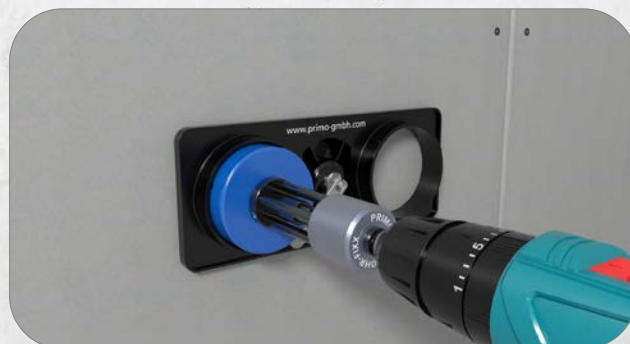
3. For multiple combinations, insert the Drilling Template into the first hole. Align using the integrated spirit level and tighten the lever. Drill more holes with the standardized combination spacing of 71 mm by moving the Drilling Template.
