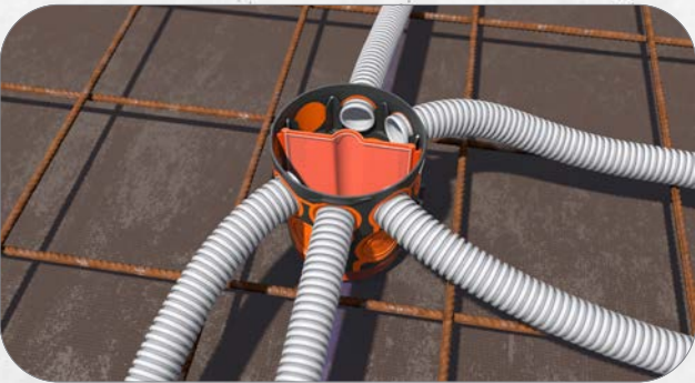
3. Insert cables or (rigid) conduits M40 without tools. Reliable strain relief due to conduit grip. Optional Divider web for two isolated circuits in one box.
