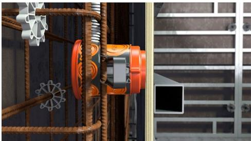
Flexible wings adapt to the respective concrete cover. Concrete covers between 20-40mm or 40-60mm.
