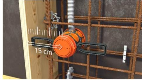
Wall mounting: With wings wings provide 15cm standard distance to door formwork. They can be rotated 180° for different concrete coverings.
