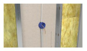
Stick the bottom part of the box with the adhesive surface onto the drywall and insert the cables or pipes.
