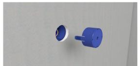
Mill out the hole with the can cutter and remove the drill cover. Snap in the upper part of the box flush with the plaster.
