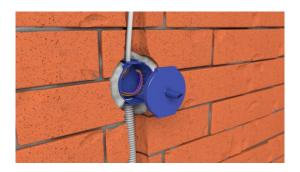
Mill the drill hole for the base of the box. Position the bottom part of the box flush, insert cables and pipes. Fit the drill cover (P003) onto the base of the box.
